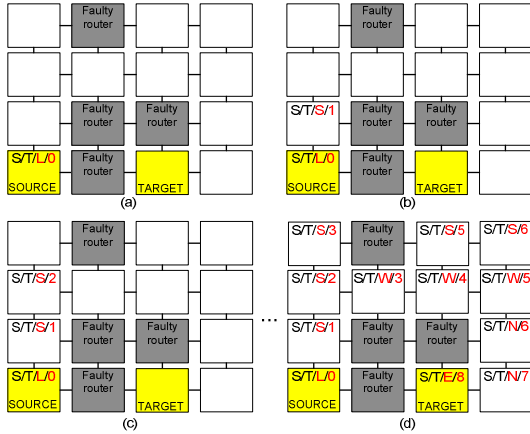
Figure 3 – Seek steps of the method in a 4x4 mesh, with four faulty routers.
