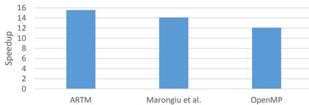
Fig. 9. Strassen algorithm speedup comparison for  $64 \times 64$  matrices on 16 cores (ARTM vs. prior art in [9])
