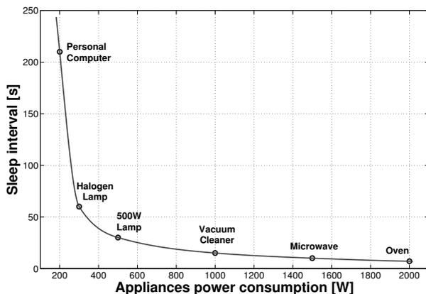
Fig. 4. Optimized sustainability curve. For a given appliance power consumption the curve returns the minimum sleep time interval to guarantee sustainable operations
