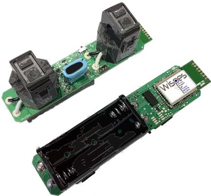
Fig. 3. Top and bottom view of the WCSN hardware prototype used in laboratory test.
