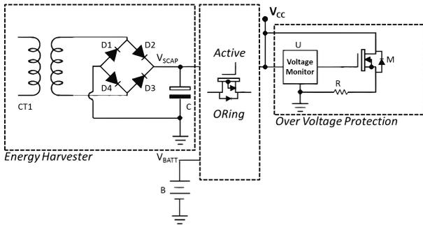
Fig. 2. Power supply schematic of the wireless current sensor node. A low-loss, low-power active ORing system generates  $V_{CC}$  by selecting the suitable source between the backup battery and the energy harvester. An over voltage protection is provided to avoid MCU and radio transceiver damages.
