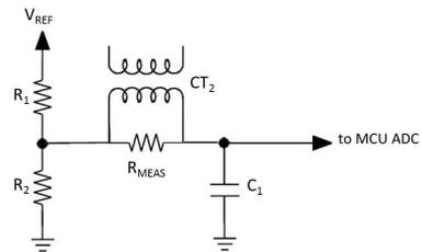
Fig. 1. Schematic of the current sensing circuit.
