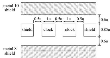
Fig. 5. Cross section of Wires in any H-tree Segment
