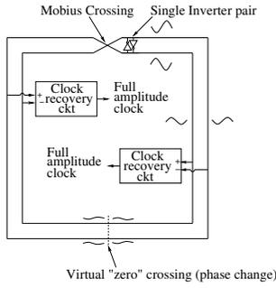
Fig. 1. Standing Wave Oscillator [13]
