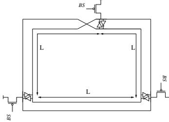
Fig. 2. Circuit Topology of a  $3\lambda/2$  SWO Ring
