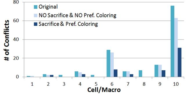
Figure 11. Number of conflicts with the fixed-area flow for the different cell and macro layouts showing the effects of using preferred coloring (see Figure 9) and the possible sacrifice of redundant contacts and M1 pin segments.
