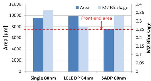
Figure 4. Total cell area and M2 blockage results for M1 patterning: 60nm pitch with SADP and 64nm with LELE DP with conservative rules to avoid conflicts compared with 80nm pitch with single-exposure 1D patterning.
