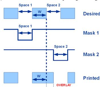
Figure 2. Example showing translation of overlay error into CD variation in negative-tone DP process.
