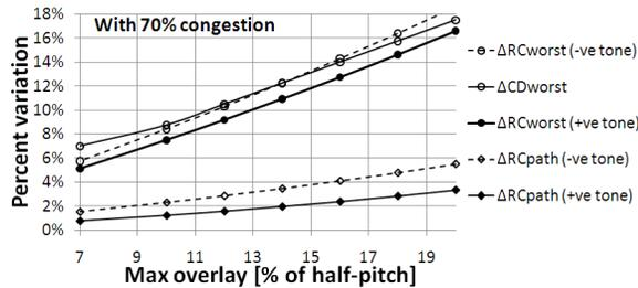
Figure 12. Plots of average and worst case CD and  $C$  variations versus requirement of maximum overlay with 70% congestion in positive and negative DPL.
