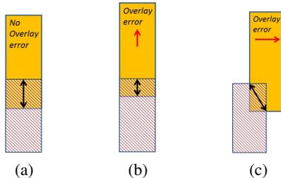
Figure 13. Example of a stitch in a vertical line (a), a possible failure with overlay error in  $Y$  direction that may occur after lineend pullback (b), and a possible failure with overlay error in  $X$  direction due to narrowing (c).
