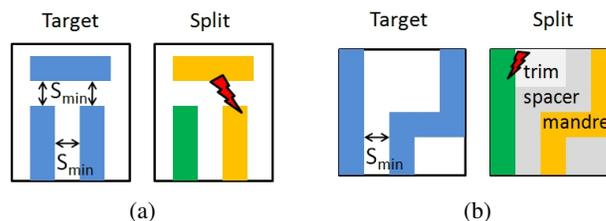
Figure 1. Examples of a LELE forbidden pattern (a) and a SADP forbidden pattern (b).  $S_{min}$  denotes the minimum spacing of single-patterning.
