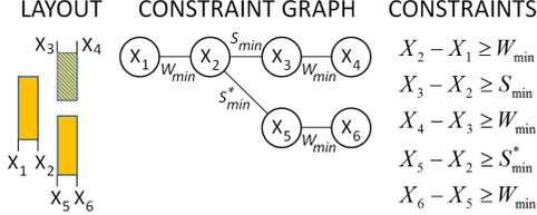
Figure 10. Example of  $x$ -direction constraint graph construction and constraint definition for a double-patterned layer.  $W_{min}$  is the minimum width rule,  $S_{min}$  is the side-to-side different-color spacing rule, and  $S_{min}^*$  is the side-to-side same-color spacing rule.
