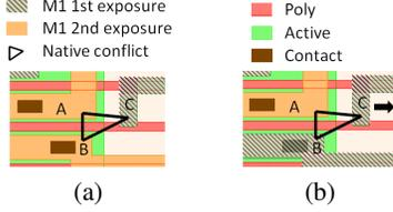
Figure 9. Layout-coloring of features of an odd cycle can affect the efficiency of conflict removal. In (a), the conflict is on M1 between shapes A and B and can only be fixed if the gates are spaced apart and area is increased; in (b), the conflict is on M1 between shapes B and C and can be fixed by moving C in the direction of the arrow without increasing area.
