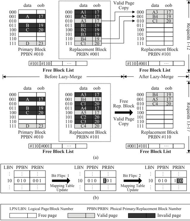
Fig. 3: Example of WAB-FTL. (a) The status variation of blocks in NAND flash memory. (b) The bit flips caused by the update of block-level mapping table in PCM.
