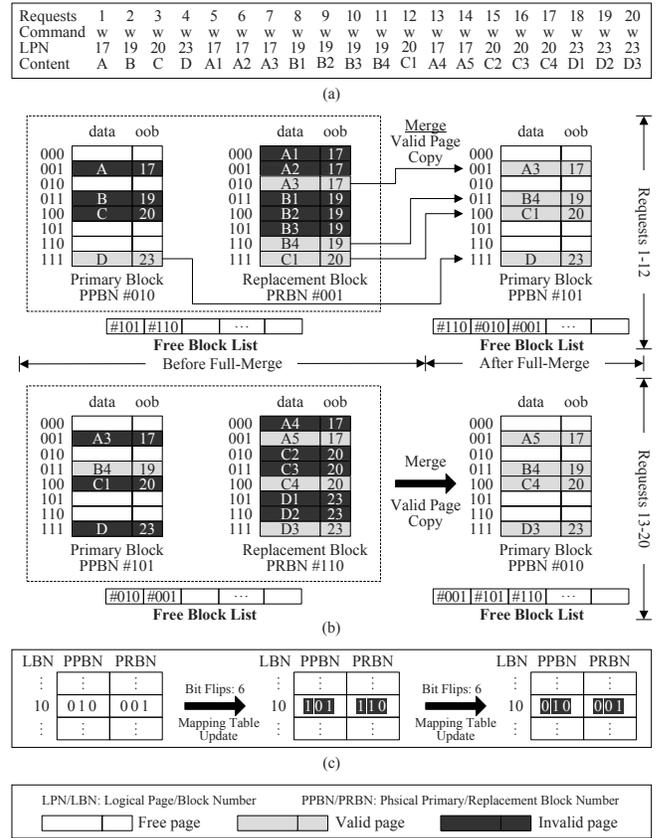
Fig. 2: Motivational example. (a) I/O access requests. (b) The status variation of blocks in NAND flash memory. (c) The bit flips caused by the update of block-level mapping table in PCM.
