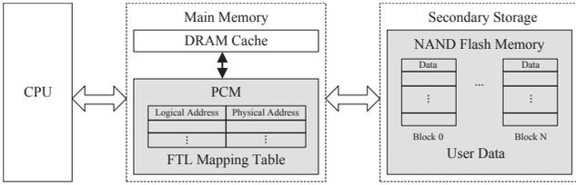
Fig. 1: PCM-based embedded system with NAND flash memory.
