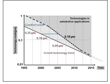
Figure 1. Overall CMOS technology trend compared to CMOS technology trend used for automotive applications
