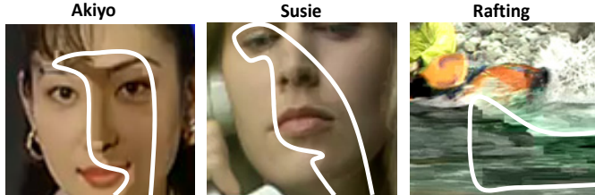
Fig. 1 Excerpts from different video sequences showing the effect of soft errors on the subjective video quality (white lines encircle the corrupted regions)
