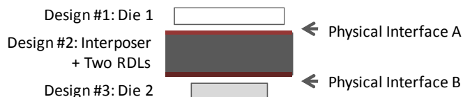
Figure 2. An integrated 3D system comprises 2D designs from three different sources.
