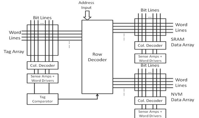
Fig. 1. Reconfigurable hybrid cache (RHC) design
