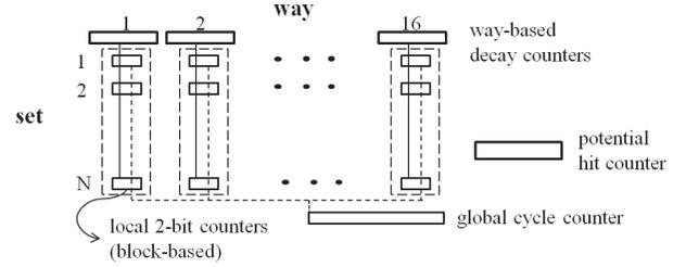
Fig. 3. Counters for dynamic reconfiguration
