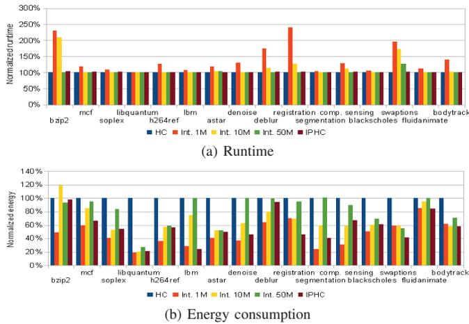
Fig. 8. Comparison of runtime and energy on two dynamic schemes
