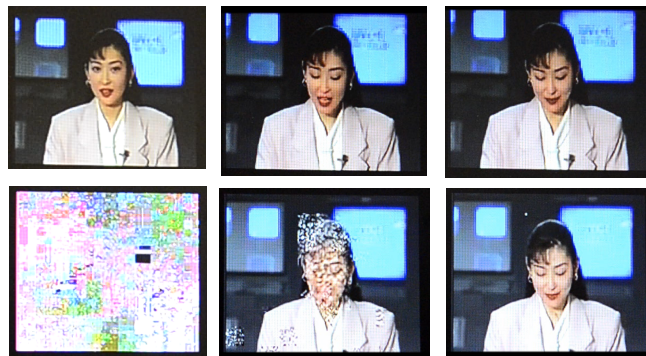
Figure 1: Dependent on the location where errors appear inside the circuit the visual quality of the decoded video is affected differently
